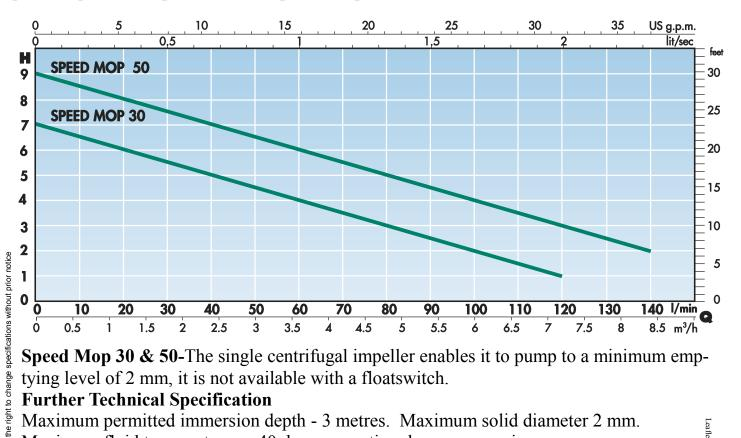
Speed Mop 30 & 50-The single centrifugal impeller enables it to pump to a minimum emptying level of 2 mm, it is not available with a floatswitch.
